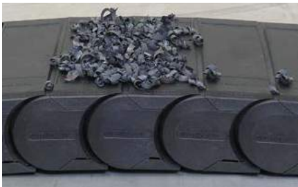
Example: Cover system with chips
