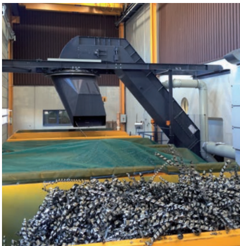
Delenie triesok a rozdelenie na deličke. Chip separation and distribution on a peeling machine.
